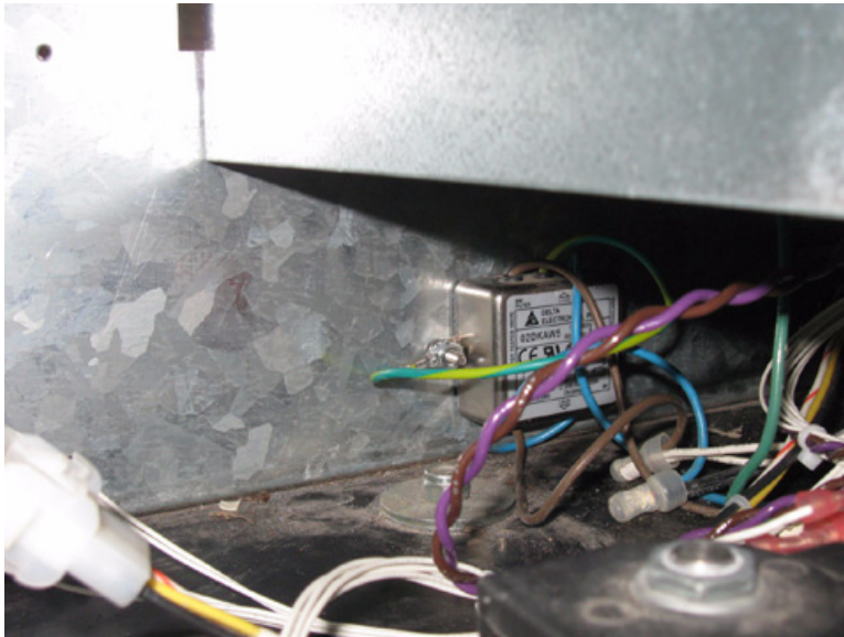
Filter viewed from opposite side. From this view, the screw to be removed is out of view on the right side of filter. The ground wire may be attached to either screw.
